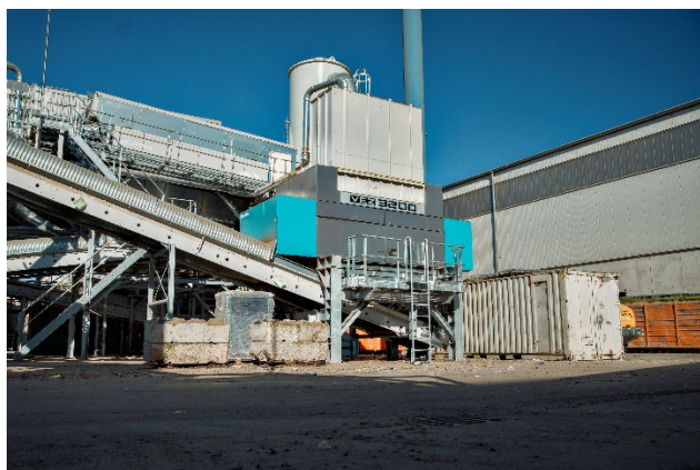
Caption 1: The VEZ 3200 is equipped with two HiTorc direct drives to ensure precise control of the particle size of the output material.
