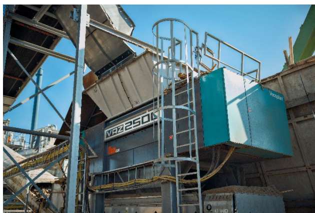
Caption 2: The VRZ 2500 handles primary shredding and takes care of a large part of the work at the start of the line, thereby reducing the load on the downstream units and keeping the line running smoothly.
