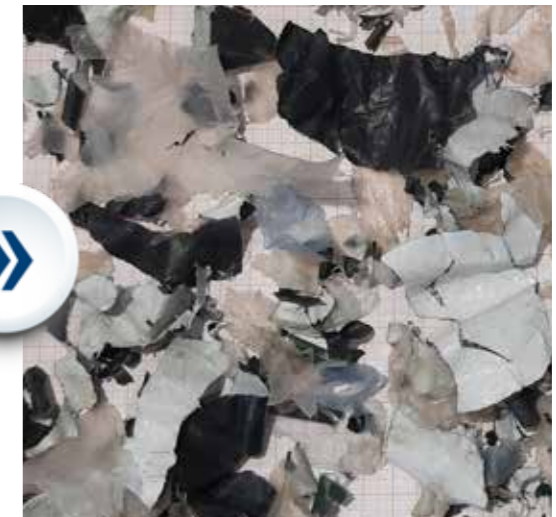
Dry cleaning of film (LLDPE), origin: agriculture (silobale wrapping film)
