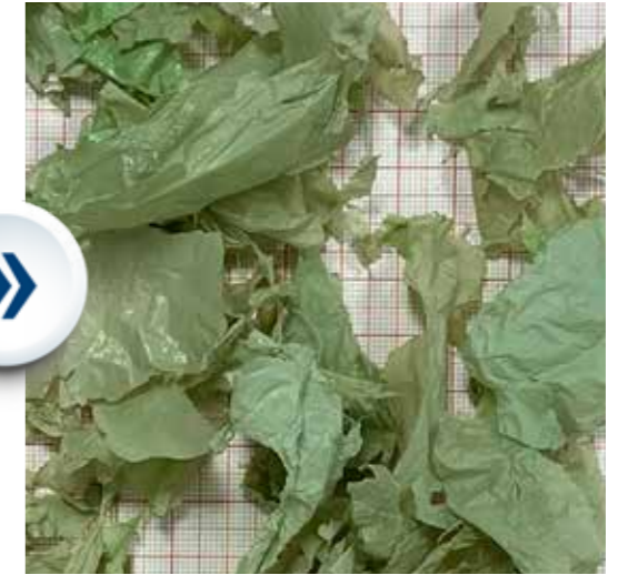
Dry cleaning of film (LLDPE), origin: agriculture (silobale wrapping film)
