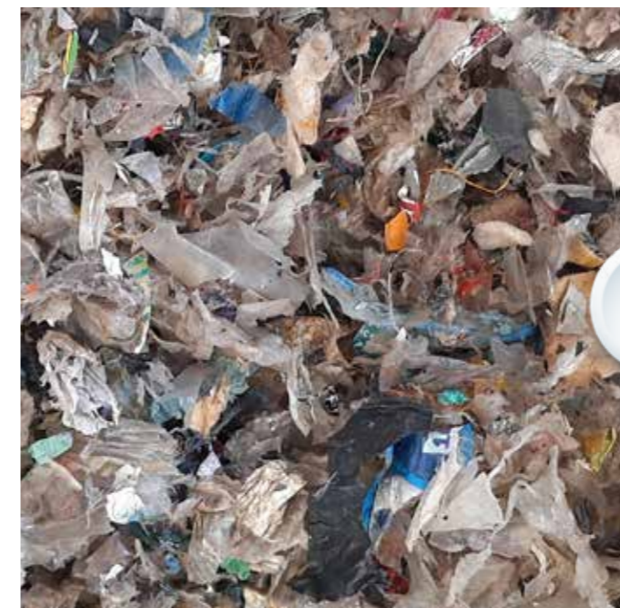
Dry cleaning of film (LDPE), origin: household waste
