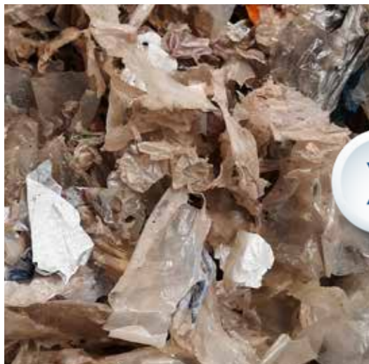
Dry cleaning of film (LDPE), origin: LVP sorting (specification DSD 310)
