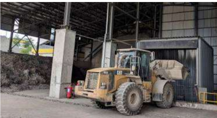
Image 3: The RDF can also be delivered to the reception station by a wheel loader.
