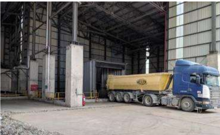
Image 2: A truck unloads RDF at a reception station with a capacity of approximately 100 m 3 .
