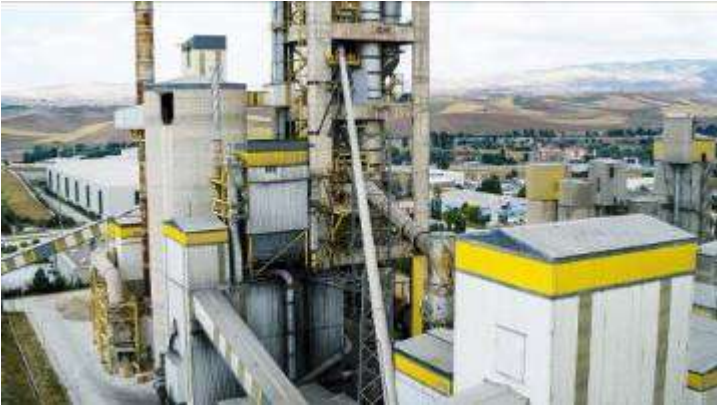
Image 1: The completely enclosed VecoBelt conveys material over long distances while protecting it from environmental influences. It can overcome inclines of up to 18°.
