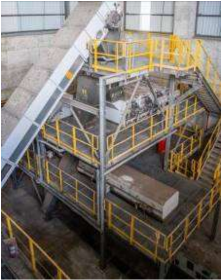
Image 4: A drum magnet extracts ferrous impurities from the mass. Following this process, the RDF passes through a disc screen to separate particles larger than 70 mm. The material is then transported on to a belt weigher.
