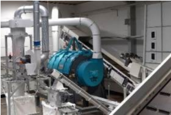
Image 2: Mechanical drying removes impurities like paper fibres, dust and organic residues. Dissolved dirt escapes as the rotor turns, while fibres and dirt are sucked off.
