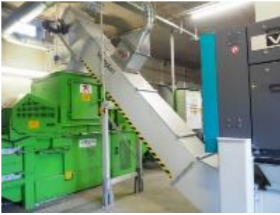
Photo 6: Vecoplan also supplied a drag chain conveyor for moving shredded material to the press.
