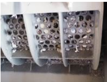
Photo 9: The necessary screen sizes can be changed in just a few minutes, depending on the security level.
