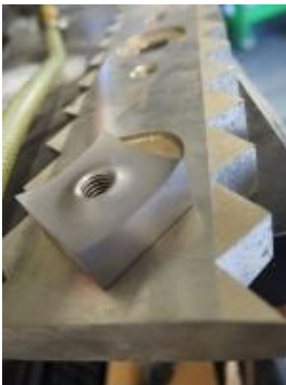
Photo 7: A cutting crown on a counter blade – both can be easily replaced and used multiple times.
