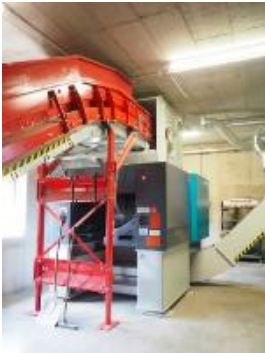
Photo 3: Files travel on the customer-facing conveyor belt (red) to the Vecoplan shredder.
