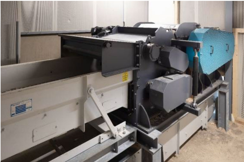
Photo 2: The Vecoplan VTH 250-850 drum chipper produces high-quality wood chips for downstream processing.
