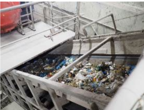
Photo 8: The conveyor system transports the shredded output out of the machine.
