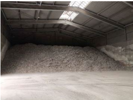
Photo 11: Dry stabilate is a very efficient refuse-derived fuel (RDF).
