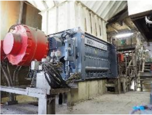
Photo 4: The powerful VVZ 2500 has been in use for pre-shredding since 2008. It achieves a very high level of efficiency, thanks to its HiTorc direct drive (in red).
