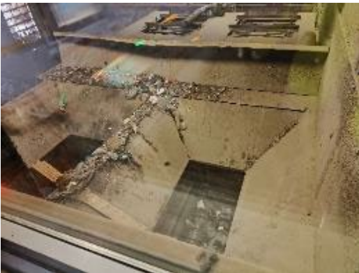
Photo 5: The VVZ is fed via the filling hopper.
