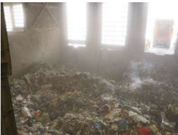
Photo 3: The wet waste consisting of wood, paper, textiles and plastics as well as all kinds of extraneous materials is collected in a deep bunker.
