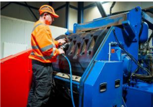
Photo 5: An optimal maintenance plan is an essential part of new machine design. The aim is to make repeated operations such as knife replacement faster and easier.
