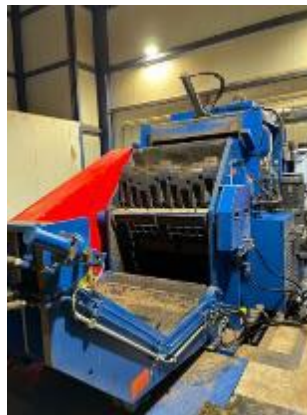
Photos 4 a +b: The VVB primary crusher features a robust design. A service platform integrated in the panel opens at an ideal height for maintenance personnel.
