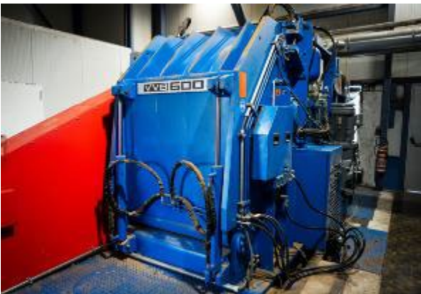
Photos 4 a +b: The VVB primary crusher features a robust design. A service platform integrated in the panel opens at an ideal height for maintenance personnel.
