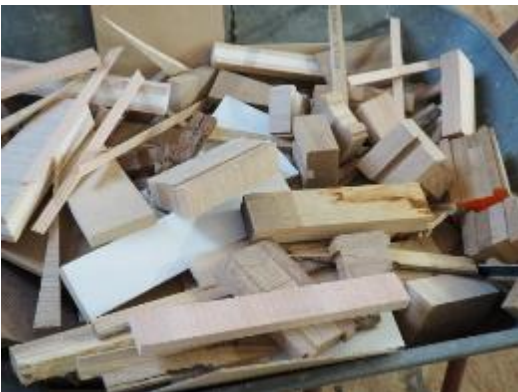
Photo 5: Untreated residual wood and old wood generated during production is fed into the furnace and used for heating.
