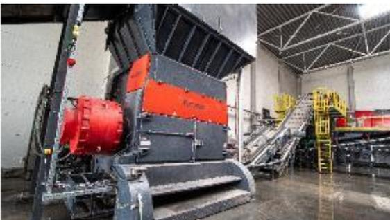
**Image 3:** The VEZ 2500 TV with its high-torque drive handles the pre-shredding. A connected conveyor belt transports the material to the following processing stage.
