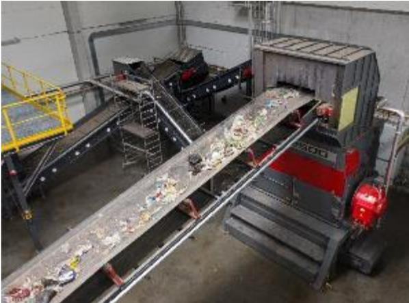
**Image 4:** The VEZ 2500 TT shreds the challenging materials into a homogeneous output, which is then used as RDF.
