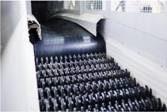
Photo 4: The star screening machine separates excess lengths from the material.
