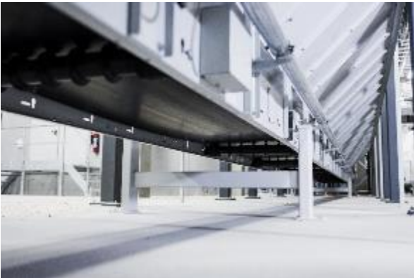
Photo 2: The waste wood falls directly from the sawmill onto the conveyor system, ready for the next stage of pellet production.
