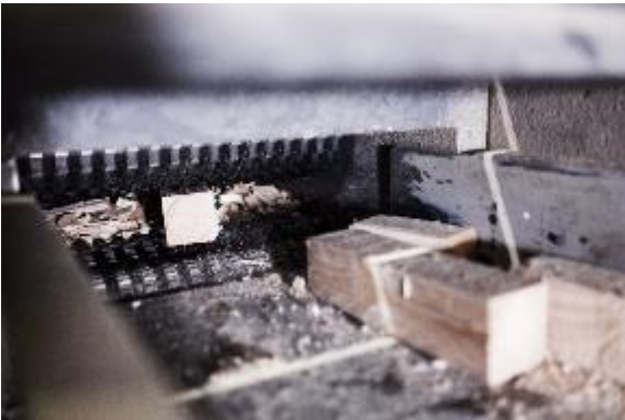
Photo 5: The screened excess lengths and offcuts from the board sorting are transported to the drum chipper via belts and vibrating conveyors.
