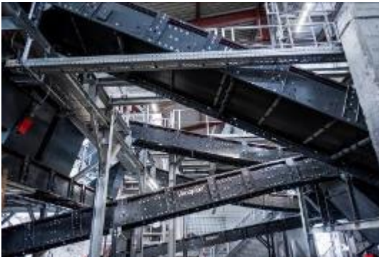
Photo 4: Vecoplan supplied all of the conveyor equipment: trough conveyors, pendulum distributors, chain conveyors and double worm conveyors.
