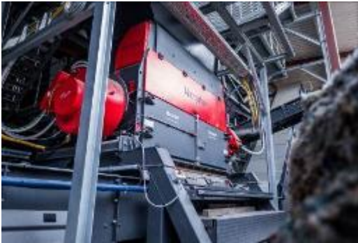
Photo 3: For post-shredding Vecoplan installed the VEZ 2500 TT, which is equipped with a high-performance cutter designed for maximum throughput.
