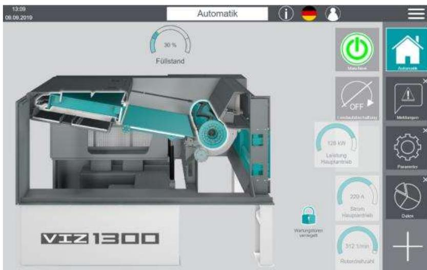
**Image 2:** Vecoplan has designed the new control panel in such a way that all the work processes at the shredders can be handled intuitively by the employees, who can also go online via the control panel.
