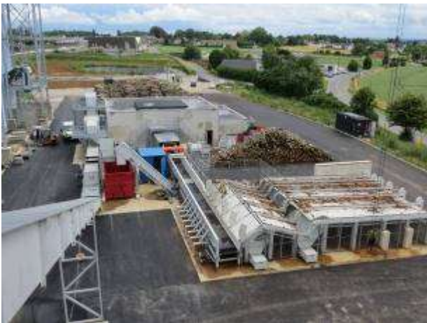
Image 3: Vecoplan biomass chippers are elementary aggregates in the processing of biomass in biomass heat & power plants.
