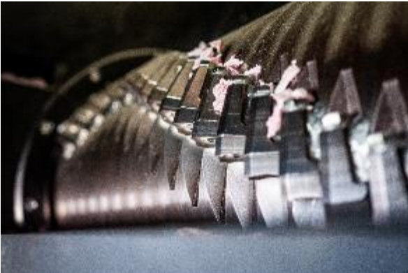
Photo 5: The cutting geometry is exceptionally flexible. Vecoplan can adapt the system's performance to input and output requirements through individual rotor and blade configurations and the choice of the relevant screen.
