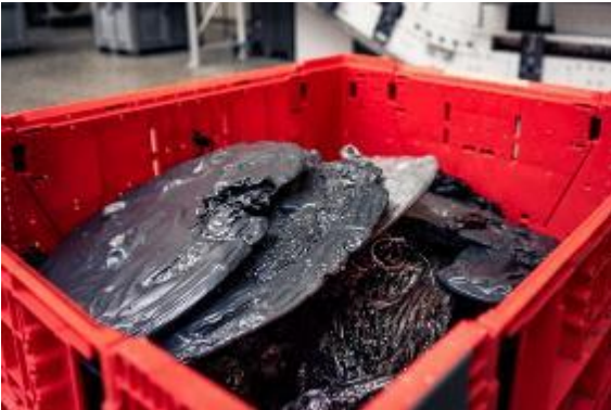
Photo 2: The input material includes purgings (post-industrial waste) ...
